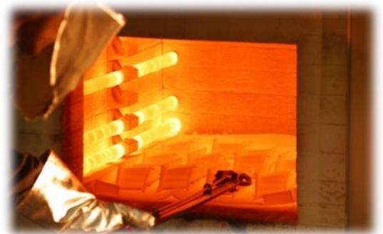
Figure 1. Furnaces used in heat treatment applications require accurate and reliable control system performance.
